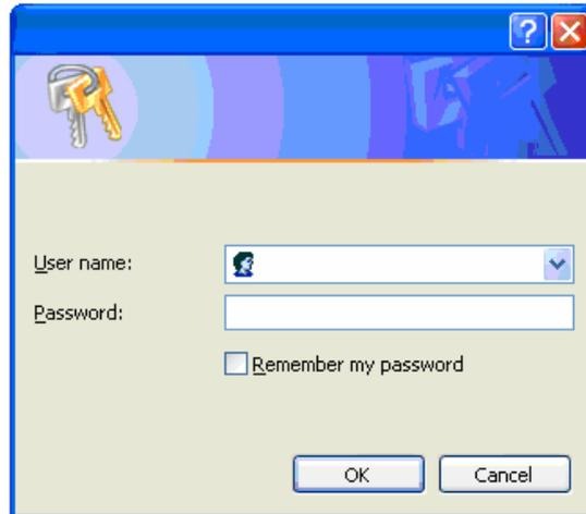
2. Please input username and password in the field respectively. Default username is 'admin' and default password is 'admin', then press **<OK>** button. Once the login details are entered correctly, users can see the web management interface of this modem router.
