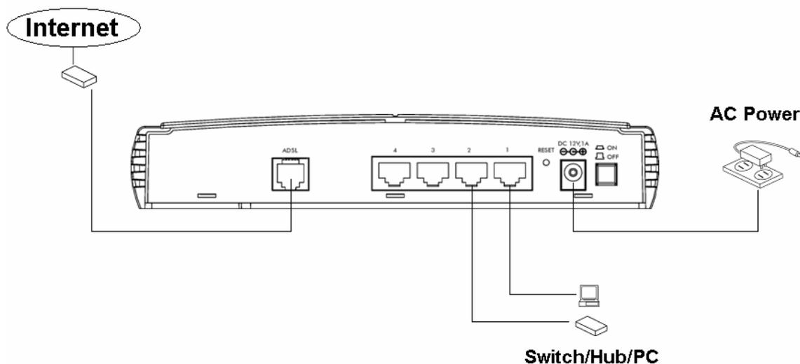
**Step 1.** Connect the ADSL port of modem router by telephone cable (RJ-11) to an outlet or splitter.
