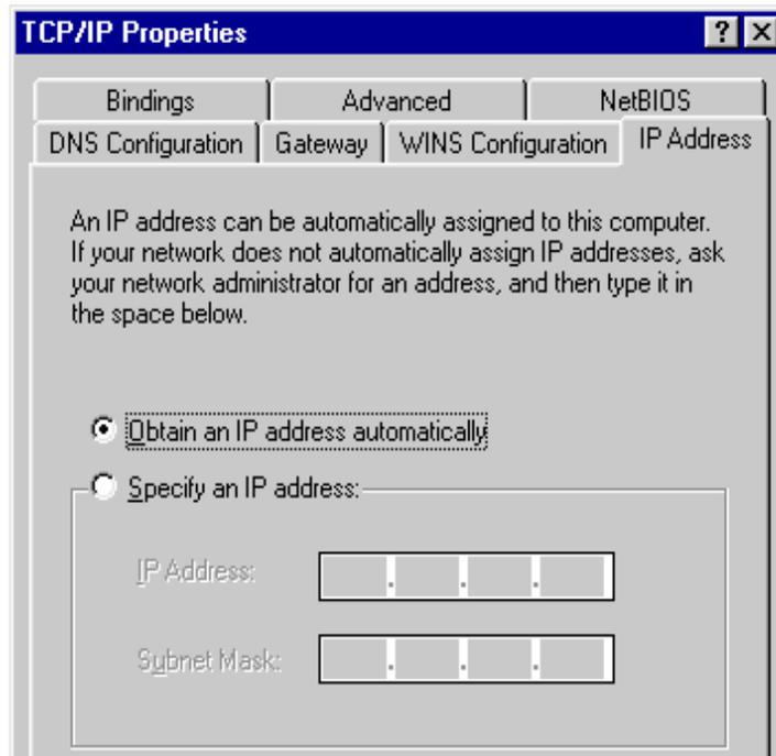
8. Reboot the PC. PC will now obtain an IP address automatically from the Broadband Router's DHCP server.
