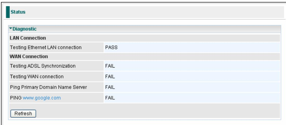
The screenshot shows a web interface with a 'Status' tab selected. Below it, the 'Diagnostic' section is expanded, showing a table with the following data:
