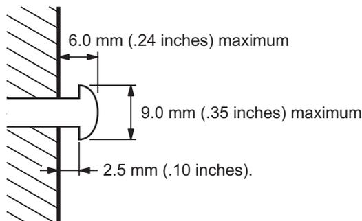
There must be .10 inches (2.5 mm) between the wall and the underside of the screw head.
