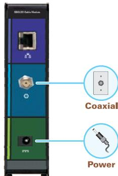
4. Plug the power cord into the electrical outlet. This turns on the SB6120. You do not need to unplug it when not in use. The first time you plug in the SB6120, allow it 5 to 30 minutes to find and lock on the appropriate communications channels.
