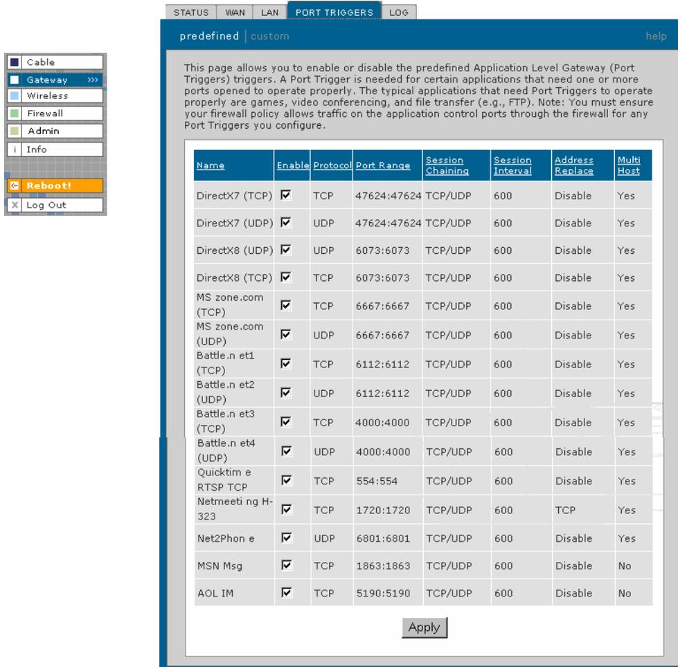
This page allows you to enable or disable the predefined Application Level Gateway (Port Triggers) triggers. A Port Trigger is needed for certain applications that need one or more ports opened to operate properly. The typical applications that need Port Triggers to operate properly are games, video conferencing, and file transfer (e.g., FTP). Note: You must ensure your firewall policy allows traffic on the application control ports through the firewall for any Port Triggers you configure.
