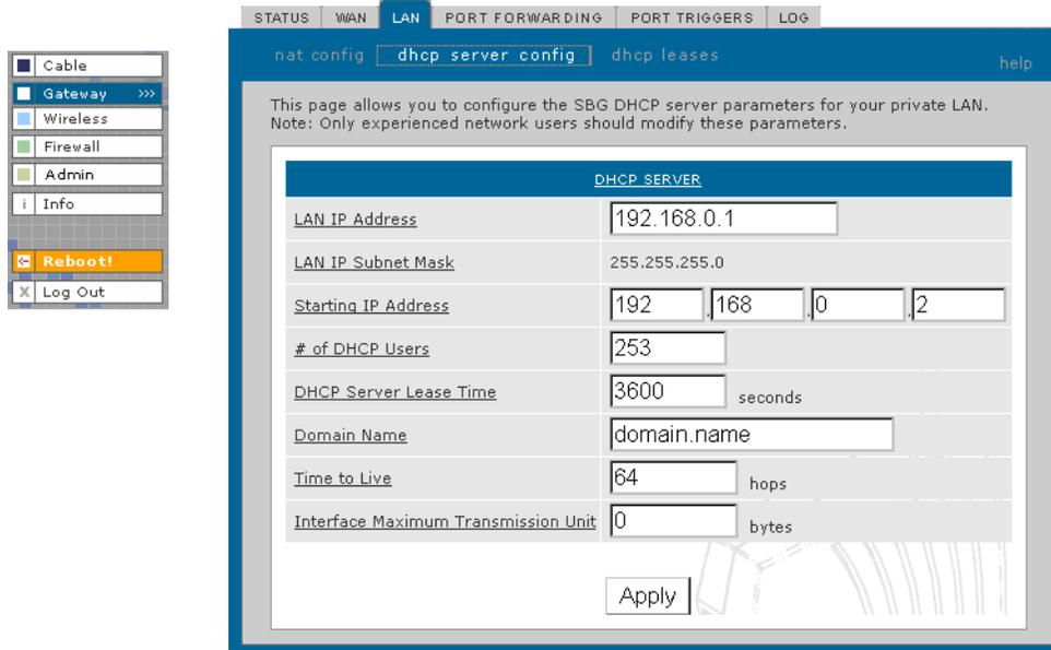
The screenshot shows the DHCP server configuration page. The left sidebar contains navigation options: Cable, Gateway (selected), Wireless, Firewall, Admin, Info, Reboot!, and Log Out. The main content area has tabs for STATUS, WAN, LAN (selected), PORT FORWARDING, PORT TRIGGERS, and LOG. The DHCP server configuration form includes the following fields:
