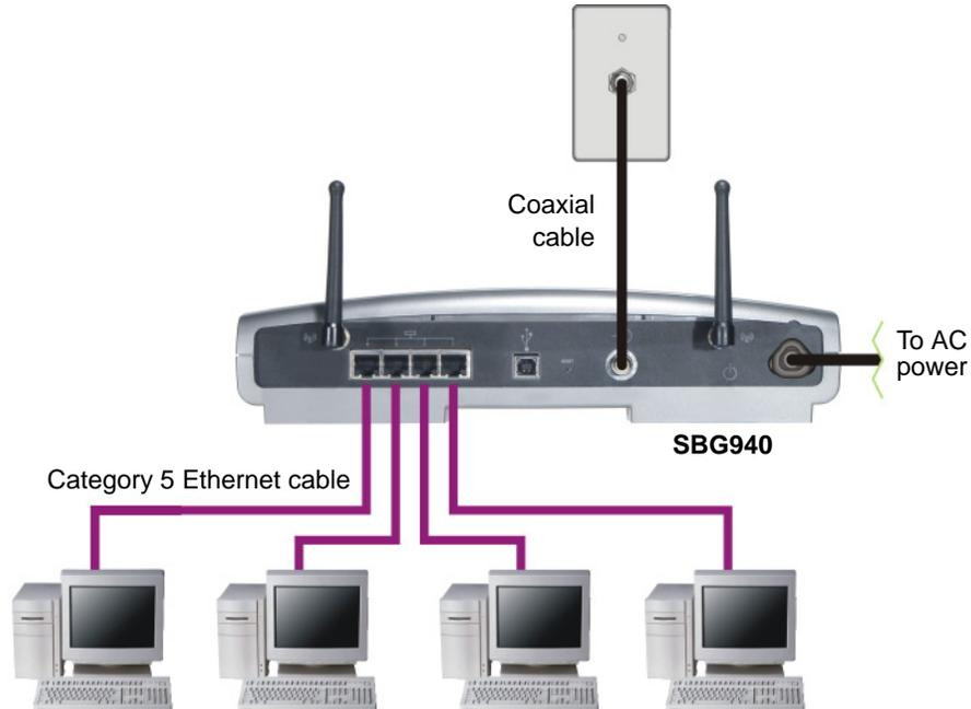
A wired Ethernet LAN with more than four computers requires one or more [hubs](#), [switches](#), or [routers](#). You can:
