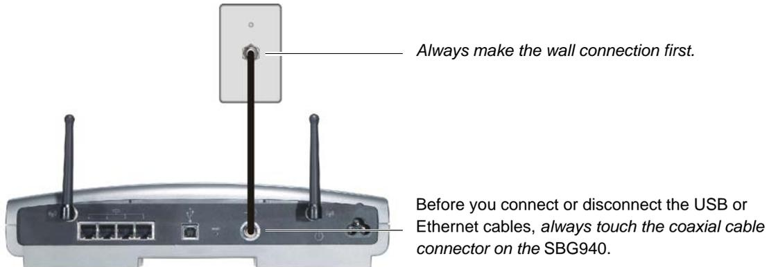
To avoid potential shock, always unplug the power cord from the wall outlet or other power source before disconnecting it from the SBG940 rear panel.
