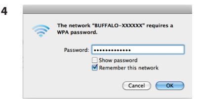
Enter the value for the KEY that was noted in step 1 into the Password entry box, insert a check mark into [Remember this network], and click [OK].
