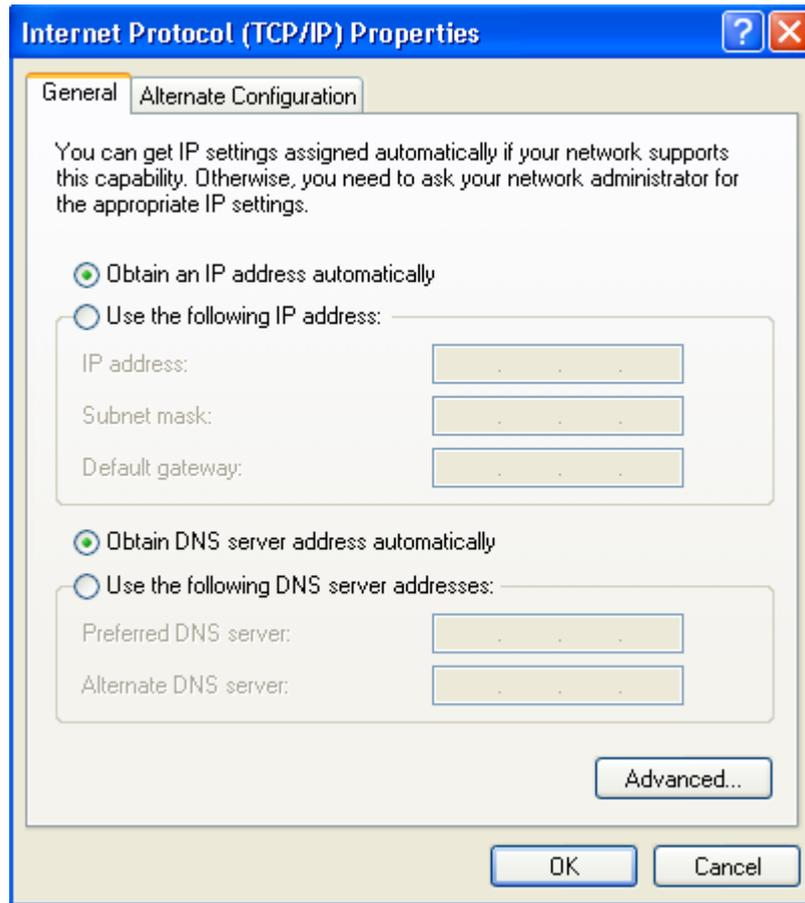
After you have successfully got an IP, please access the router by typing <http://192.168.1.1> to configure the router. (If you have changed the route's IP address, please type <http://<the new IP address of the gateway>>.)
