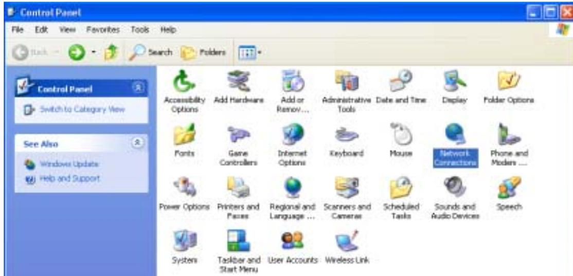
2. Select the Local Area Connection icon for the applicable Ethernet adapter (usually it is the first Local Area Connection listed). Double-click the Local Area Connection. Click the Properties button.
