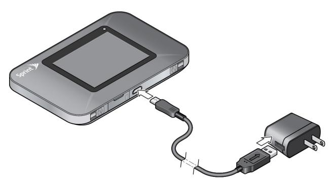
1. Insert the larger (Type A) end of the micro-USB cable into the AC charger.
