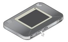
2. Remove the existing SIM card (if present) — push the SIM card in to unlock it, then pull it out of the slot.
