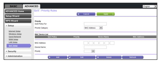
**4.** If the device is the MAC Device List, select its radio button.
