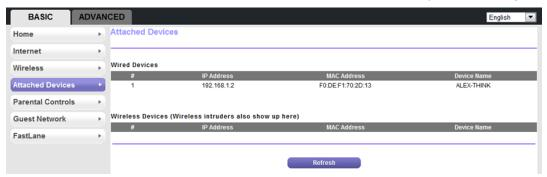
Wired devices are connected to the router with Ethernet cables. Wireless devices have joined the wireless network. NETGEAR genie displays the following information about devices that are currently connected to your network:
