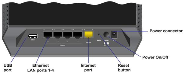
The back panel has the connections shown in the following figure.
