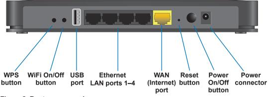
Figure 2. Router rear panel
