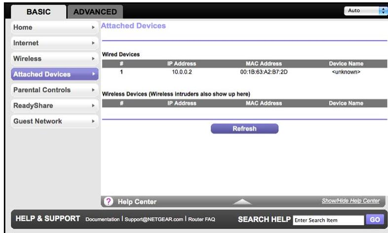
Wired devices are connected to the router with Ethernet cables. Wireless devices have joined the wireless network.
