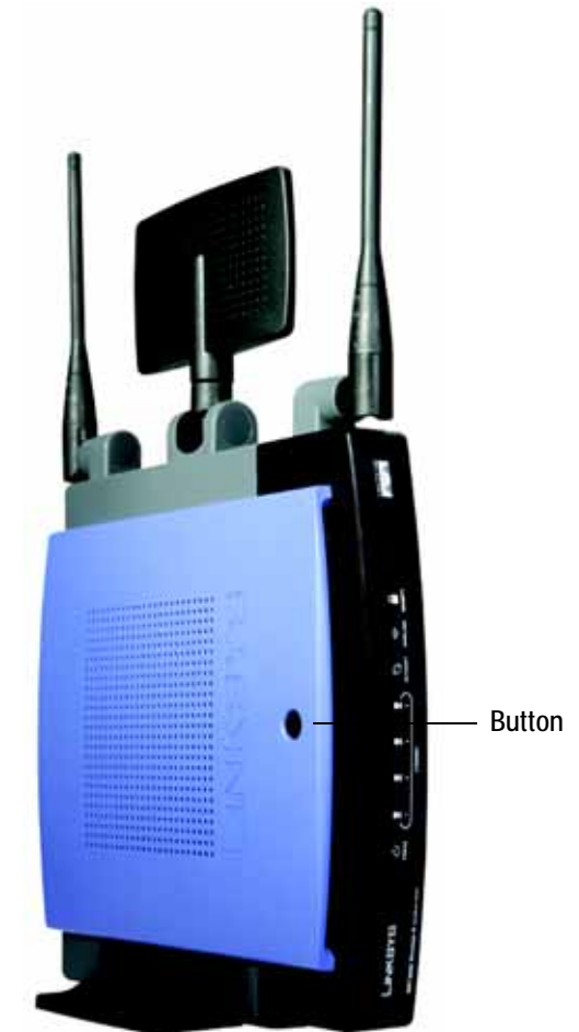
Figure 3-3: The Router's Top Panel
