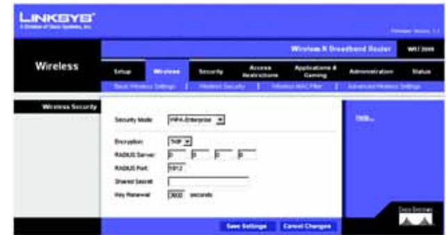
Figure 5-18: Wireless Security - WPA-Enterprise
