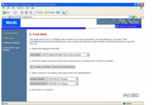
This page allows you to configure the local time zone and automatic time maintenance. Automatic time maintenance synchronizes the router with a public time server on the Internet.
