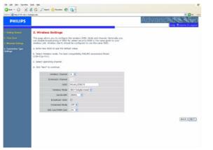
In step 2 you can change the Wireless settings of the Wireless Router. For easy installation it is advised to keep the default settings. If you later would like to change any of the wireless settings you can do so via the menu in the Wireless Router.
