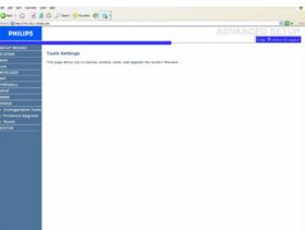
Use the Maintenance menu to backup the current configuration, restore a previously saved configuration, restore factory settings, update firmware, and reset the Wireless Router.
