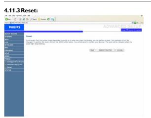
Click "REBOOT ROUTER" to reset the Wireless Router. If you perform a reset from this page, the configuration will not be changed back to the factory default settings.
