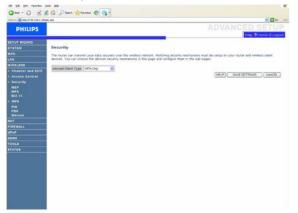
The router can transmit your data securely over the wireless network. Matching security mechanisms must be setup on your router and wireless client devices. You can choose the allowed security mechanisms in this page and configure them in the sub-pages.
