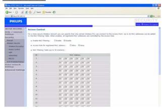
Access Control allows users to define the outgoing traffic permitted or not-permitted through the WAN interface. The default is to permit all outgoing traffic.
