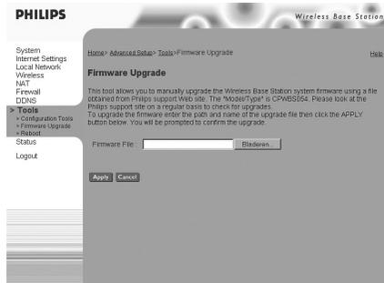
Use this screen to update the firmware or user interface to the latest versions. Download the upgrade file from the Philips web site ([www.philips.com/support](http://www.philips.com/support)) and save it to your hard drive. In the Upgrade Target field, choose Firmware. Then click Browse to look for the previously downloaded file. Click APPLY. Check the Status page Information section to confirm that the upgrade process was successful.
