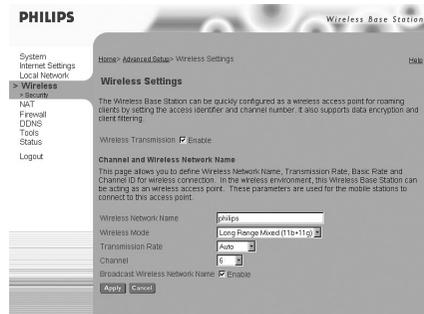
You must specify a common radio channel and Network Name (SSID) to be used by the Wireless Base Station 11g and all of your wireless clients. Be sure you configure all of your clients to the same values. Network name (SSID). This should be set to the same value as other wireless devices in your network. (Default: philips.)
