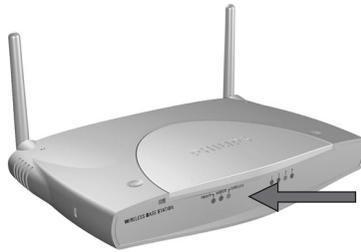
Observe the 'power', 'wireless', and 'modem' LEDs on the front of the Wireless Base Station 11g lighting up constantly while keeping the reset button pressed for at least five seconds.
