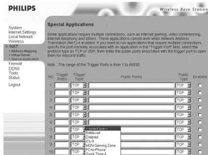
Specify the public port number normally associated with an application in the Trigger Port field. Set the protocol type to TCP or UDP, then enter the ports that the application requires.
