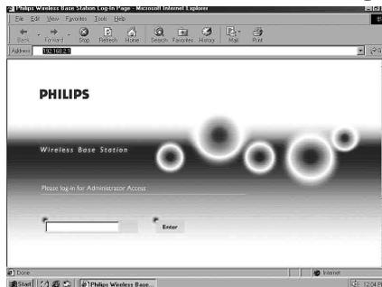
Go to configuration menu of the Wireless Base Station 11g by entering its IP address (default 192.168.2.1 into the Address Bar of your Internet browser program).
