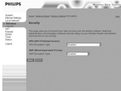
You may automatically generate encryption keys or manually enter the keys. For automatic 64-bit security, enter a passphrase and click Generate. Four keys will be generated (as shown below). Choose a key from the drop-down list or accept the default key. Automatic 128-bit security generates a single key.
