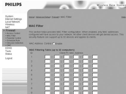
The MAC Filtering feature of the Wireless Base Station 11g allows you to control access to your network to up to 32 clients based on the MAC (Media Access Control) address of the client machine. This ID is unique to each network adapter. If the MAC address is listed in the table, that client machine will have access to the network.
