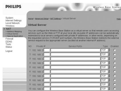
If you configure the Wireless Base Station 11g as a virtual server, remote users accessing services such as web or FTP at your local site via public IP addresses can be automatically redirected to local servers configured with private IP addresses. In other words, depending on the requested service (TCP/UDP port number), the Wireless Base Station 11g redirects the external service request to the appropriate server (located at another internal IP address).
