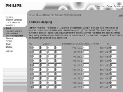
Allows one or more public IP addresses to be shared by multiple internal users. Enter the Public IP address you wish to share into the Global IP field. Enter a range of internal IPs that will share the global IP.
