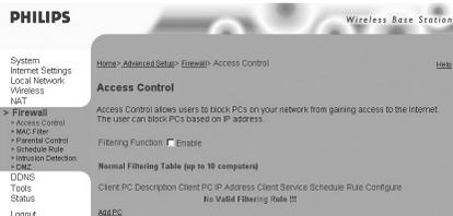
Using this option allows you to specify different privileges based on IP address for the client PCs.
