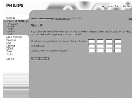
If your Internet Service Provider has assigned a fixed IP address, enter the assigned address and subnet mask for the Wireless Base Station 11g, then enter the gateway address of your ISP.
