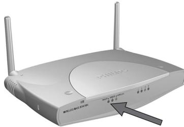
Release the reset button and observe the LEDs on the front of the Wireless Base Station 11g.
