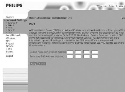
Domain Name Servers map numerical IP addresses to the equivalent domain name (e.g., www.philips.com). Your ISP should provide the IP address of one or more domain name servers. Enter those addresses in this screen.
