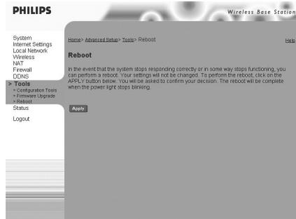
Click APPLY to reboot the Wireless Base Station. The reboot will be complete when the power LED stops blinking.
