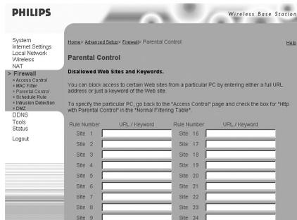
Use the above screen to block access to web sites or to web URLs containing the keyword specified in the table. containing the keyword specified in the table.
