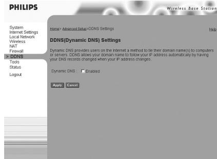
Domain Name is a series of alphanumeric strings separated by periods that maps to the address of a network connection and identifies the owner of the address.
