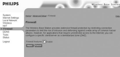
The Wireless Base Station 11g firewall can provide access control of connected client PCs, block common hacker attacks, including IP Spoofing, Land Attack, Ping of Death, IP with zero length, Smurf Attack, UDP port loopback, Snork Attack, TCP null scan, and TCP SYN flooding. The firewall does not significantly affect system performance, so we advise leaving it enabled to protect your network users.
