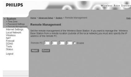
Remote Management allows a remote PC to configure, manage, and monitor the Wireless Base Station 11g using a standard web browser. Check Enable and enter the IP address of the remote host. Click APPLY.
