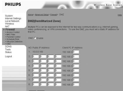
If you have a client PC that cannot run an Internet application properly from behind the firewall, then you can open the client up to unrestricted two-way Internet access. Enter the IP address of a DMZ host to this screen. Adding a client to the DMZ may expose your local network to a variety of security risks, so only use this option as a last resort.
