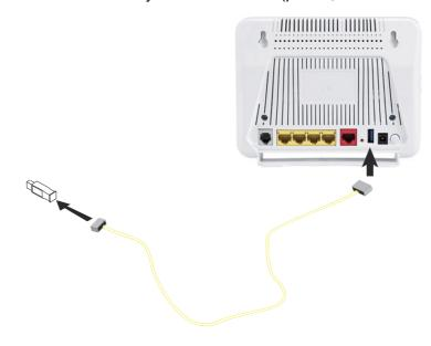
Figure 2.4 - USB Interface Connection
