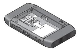
**3.** Lift the SIM card cover, remove the existing SIM card and replace it with the new one.
