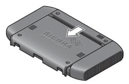
2. Slide the SIM card cover to the Open position.
