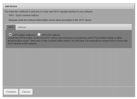
Select WPS— For WPS-enabled Wi-Fi devices or Manual—For any Wi-Fi device
