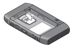
**5.** Slide the SIM card cover to the Lock position.
