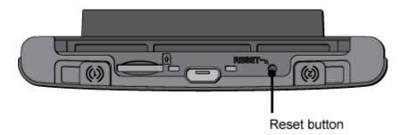
3. Insert a thin object (for example, the end of a paper clip) into the hole, and press down for about a second.
