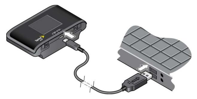
**Note:** If you'll be using USB for data transfer (and not just for charging the device), you must install the device driver (see "Windows" or "Mac", below). No installation CD is required — the device supports the TRU-Install feature.
