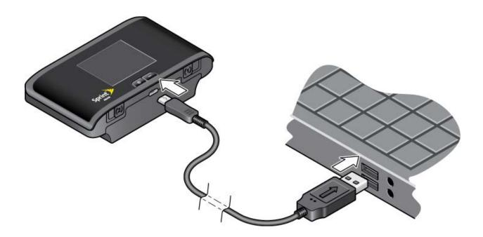
**Note:** If you'll be using USB for data transfer (and not just for charging the device), you must install the device driver. (See Making a Tethered Connection.)
