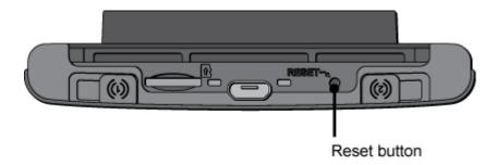
3. Insert a thin object (for example, the end of a paper clip) into the hole, and press down for five or more seconds.
