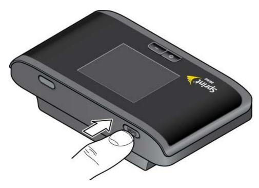
2. When the LCD of your Sierra Wireless 4G LTE Tri-Fi Hotspot displays "WPS Started", press (within 2 minutes) the WPS button on the wireless device you want to connect or select the WPS-related option in the device's software.
