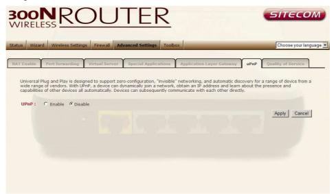
**UPnP Feature** You can enable or Disable the UPnP feature here. After you enable the UPnP feature, all client systems that support UPnP, like Windows XP, can discover this router automatically and access the Internet through this router without having to configure anything. The NAT Traversal function provided by UPnP can let applications that support UPnP connect to the internet without having to configure the virtual server sections.
