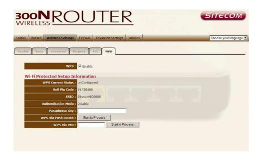
**WPS** Check the box to enable WPS function and uncheck it to disable the WPS function.
