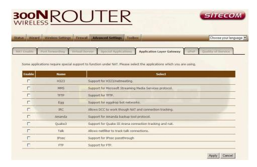
**Enable** select enable "Application Layer Gateway", then the router will let the selected application correctly pass through the NAT gateway.
