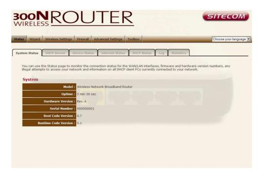
The System status section allows you to monitor the current status of your router the UP time, hardware information, serial number as well as firmware version information is displayed here.
