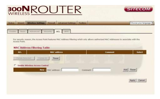
Enable wireless access control Enables the wireless access control function
