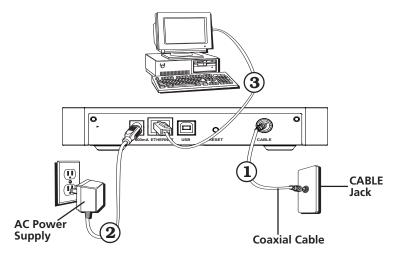
Fig. 22: Ethernet Connection
