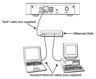
Fig. 23: Ethernet Hub Connection
