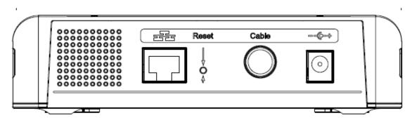
• GIGA ETHERNET: Ethernet 10/100/1000BaseT RJ-45 connector
