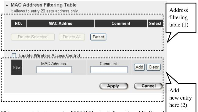
This page contains two parts of MAC filtering information. All allowed MAC addresses will be listed in upper part (1), and you can add new MAC addresses by components in lower part (2).
