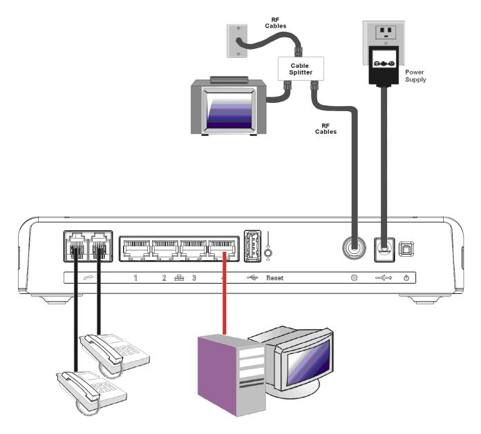
Fig. 1-7 Connect to the Modem
