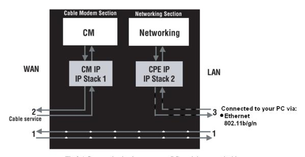
Fig.3-1 Communication between your PCs and the network side
