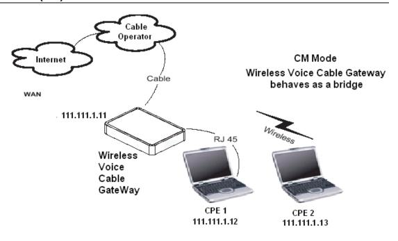
Fig. 3-2 Cable Modem Mode
