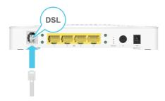
3 Plug the other end of the cable into the DSL/MODEM output port of your filter/splitter.
