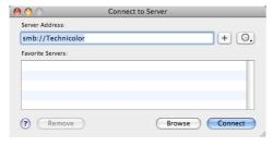
In the **Server Address** box, type **smb://<server name>**, where <server name> is the Server Name you assigned to your USB storage device (default: **smb://Technicolor**).
