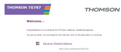
If this window does not appear browse to <a href="http://dsldevice.lan">http://dsldevice.lan</a> or to the IP address of your Thomson Gateway (by default: <a href="https://dsldevice.lan">192.168.1.254</a>) and click **Thomson Gateway** on the menu on the left-hand side.
