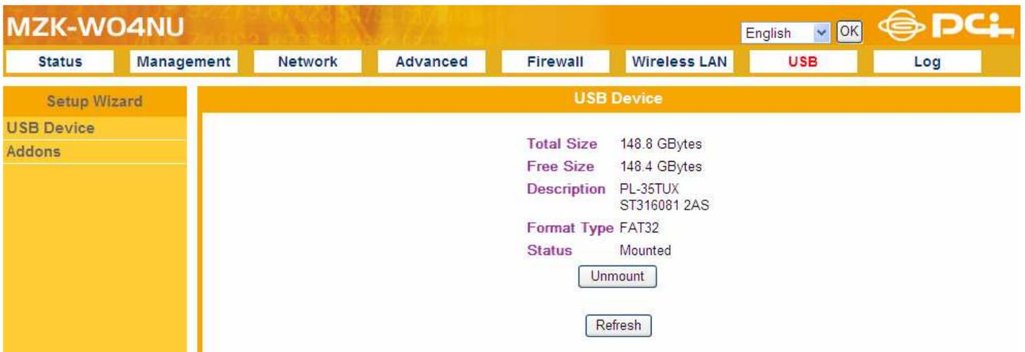
The screenshot shows the MZK-W04NU configuration interface. The top navigation bar includes 'Status', 'Management', 'Network', 'Advanced', 'Firewall', 'Wireless LAN', 'USB', and 'Log'. The 'USB' tab is selected. On the left, a 'Setup Wizard' sidebar has 'USB Device' and 'Addons' options. The main content area, titled 'USB Device', displays the following information:
