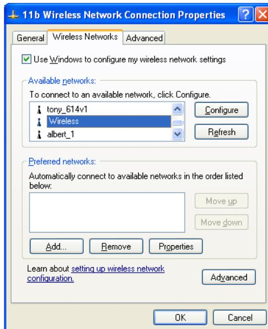
Select the SSID for the Wireless ADSL Modem Router, and click *Configure*, to see a screen like the following:
