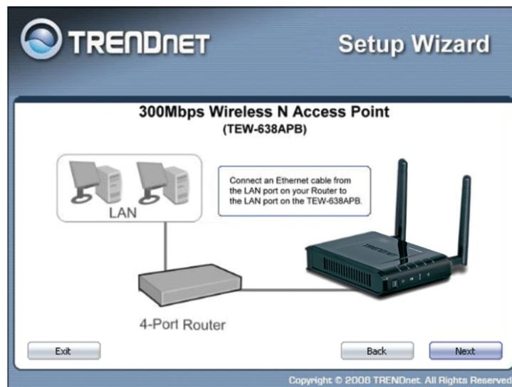
5. Plug in the power adapter of the TEW-638APB and plug in the device that will be connecting together. Verify the Power & Ethernet LEDs are light.
