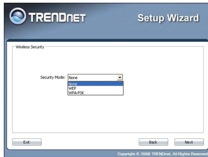
11. To use WEP security, select **WEP** and click **Next** button. Select **64-bit** or **128-bit** WEP key length, and enter your WEP key. For 64-bit encryption, enter 10 hexadecimal characters, For 128-bit encryption, enter 26 hexadecimal characters. Click **Next** to continue the setting.
