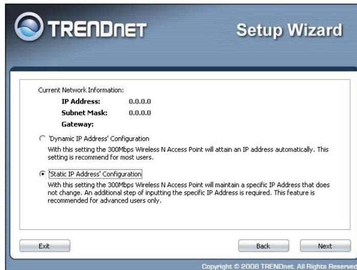
11. The default IP address is 192.168.10.100, you can choose to obtain network setting automatically, or set the IP address manually. After setting, click **Next** to complete it.
