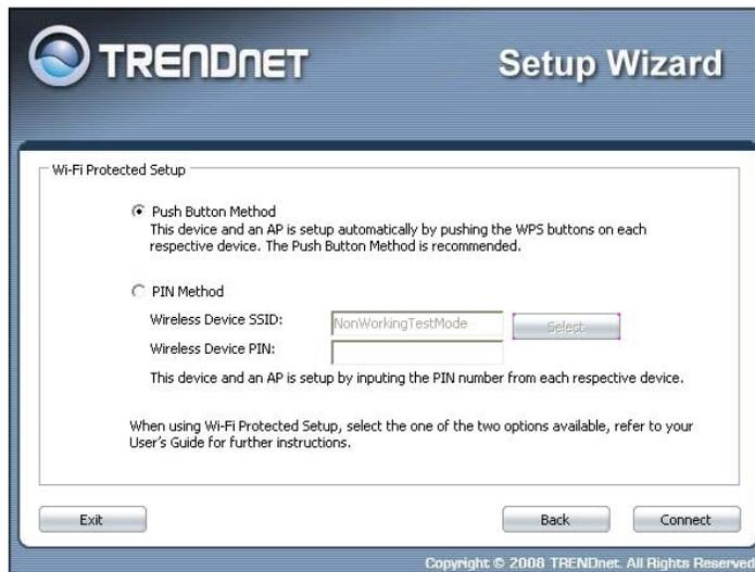
21. Use **PIN Method** and enter your wireless client PIN number on **Wireless Device PIN**, and then click **Connect** button to make wireless connection.
