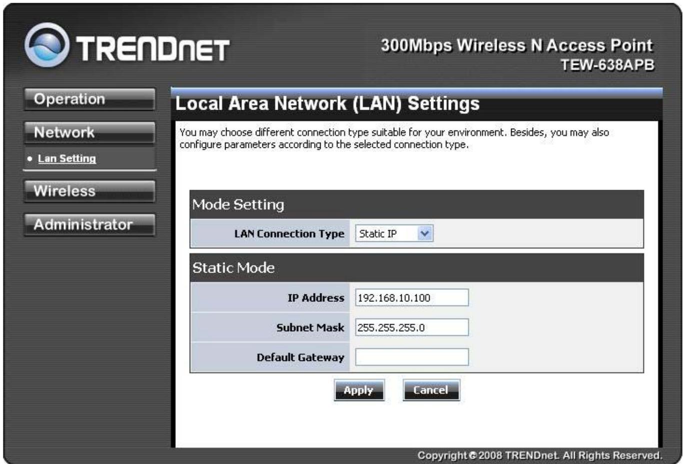
These are the settings of the LAN (Local Area Network) interface for the Access Point. The Access Point's local network (LAN) settings are configured based on the IP Address and Subnet Mask assigned in this section. The IP address is also used to access this Web-based management interface.
