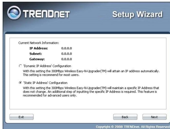
3. The default IP address is 192.168.10.100, you can choose to obtain network setting automatically, or set the IP address manually. After setting, click **Next** to continue.
