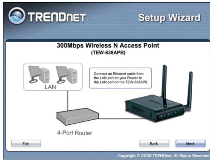
5. Plug in the power adapter of the TEW-638APB and plug in the device that will be connecting together. Verify the Power & Ethernet LEDs are light.
