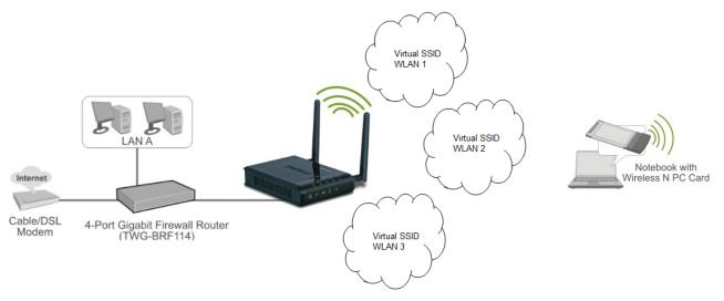
Multiple SSID (Virtual WLANs)
