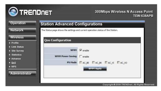
**WMM (Wireless Multi-Media)** use this feature allows wireless devices to take advantage of the wireless environment over other wireless devices.
