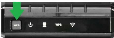
5. Once connection has been successfully established the WPS LED on the TEW-736RE will automatically turn off.
