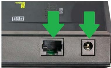
2. Connect the Power Adapter to the TEW-736RE and then to a power outlet (EU Versions will have a power button on the back. Push the power button to the "On" position). Verify that the power is on
