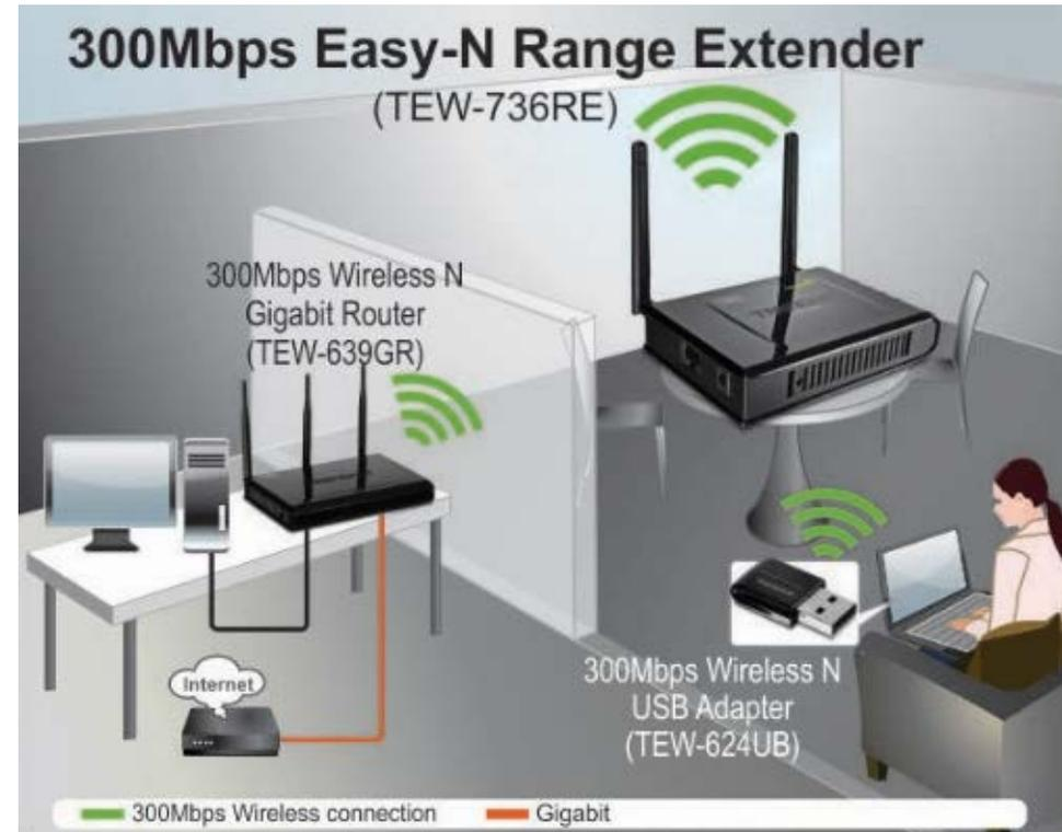
The range extender is installed in a location where the wireless signal of an existing wireless network exists. The ideal location to place the range extender is in a location where the wireless of an existing signal is available but weak. The range extender needs to detect the existing wireless signal in order to extend any signal.
