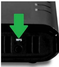
4. Press and hold the WPS button on the TEW-736RE for 5 seconds.
