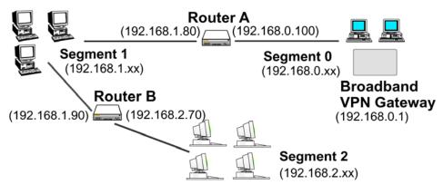
Figure 46: Routing Example
