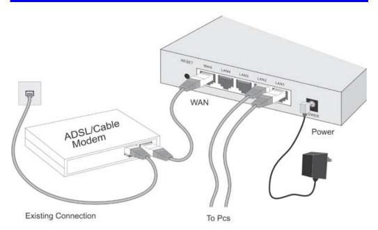
**Figure 4: Installation Diagram**
