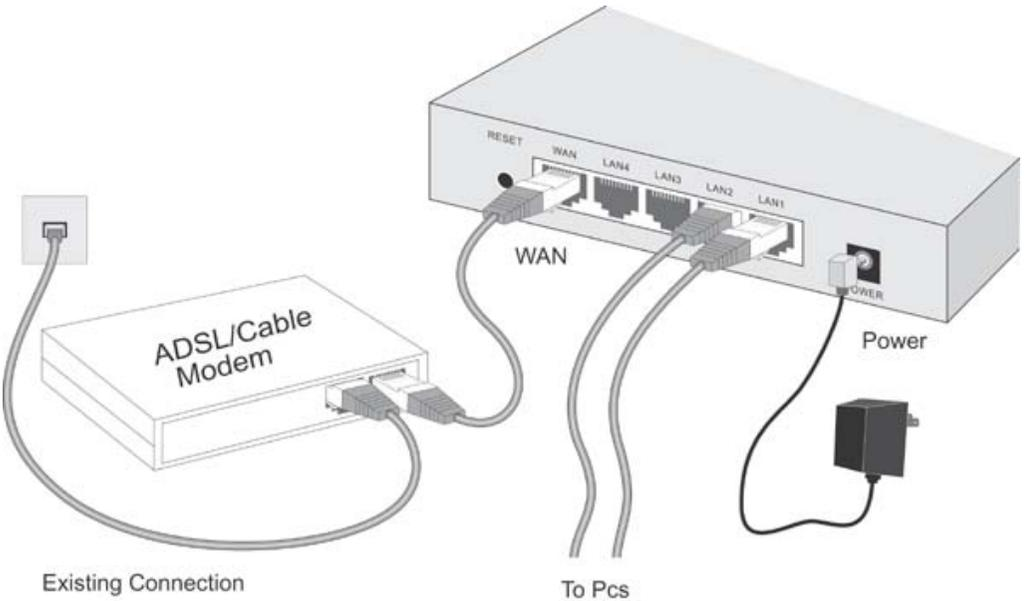
**Figure 4: Installation Diagram**
