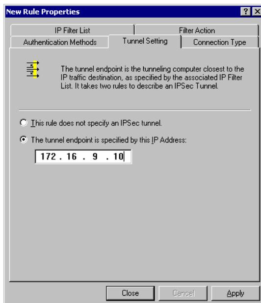
**Figure 76: Tunnel Setting**
