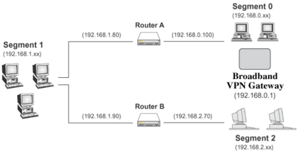
Figure 117: Routing Example
