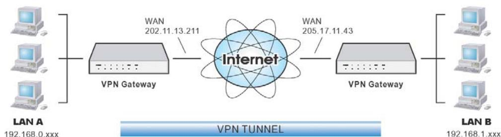
Figure 56: Connecting 2 TW100-BRV204 s
