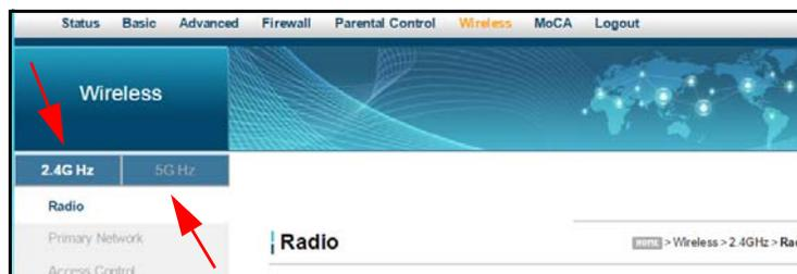
**NOTE:** Selecting the radio band as above is only an indicator of which band you are actively configuring, both the 2.4GHz and 5GHz bands are enabled by default.
