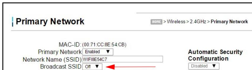
**Note:** WPS must be disabled before Broadcast SSID can be turned to **Off**.
