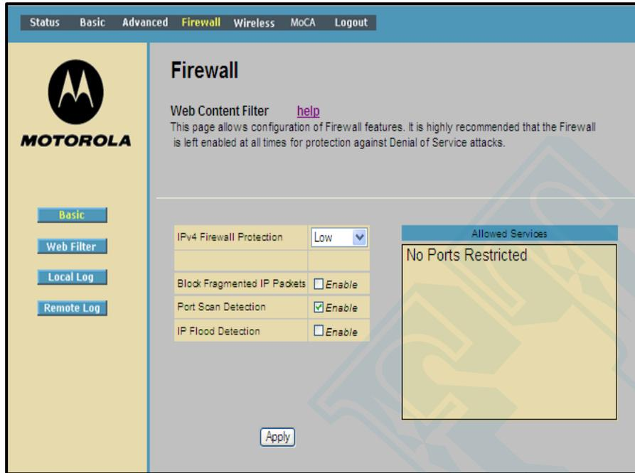
**Figure 11 – Firewall Basic Web Content Filter Page**
