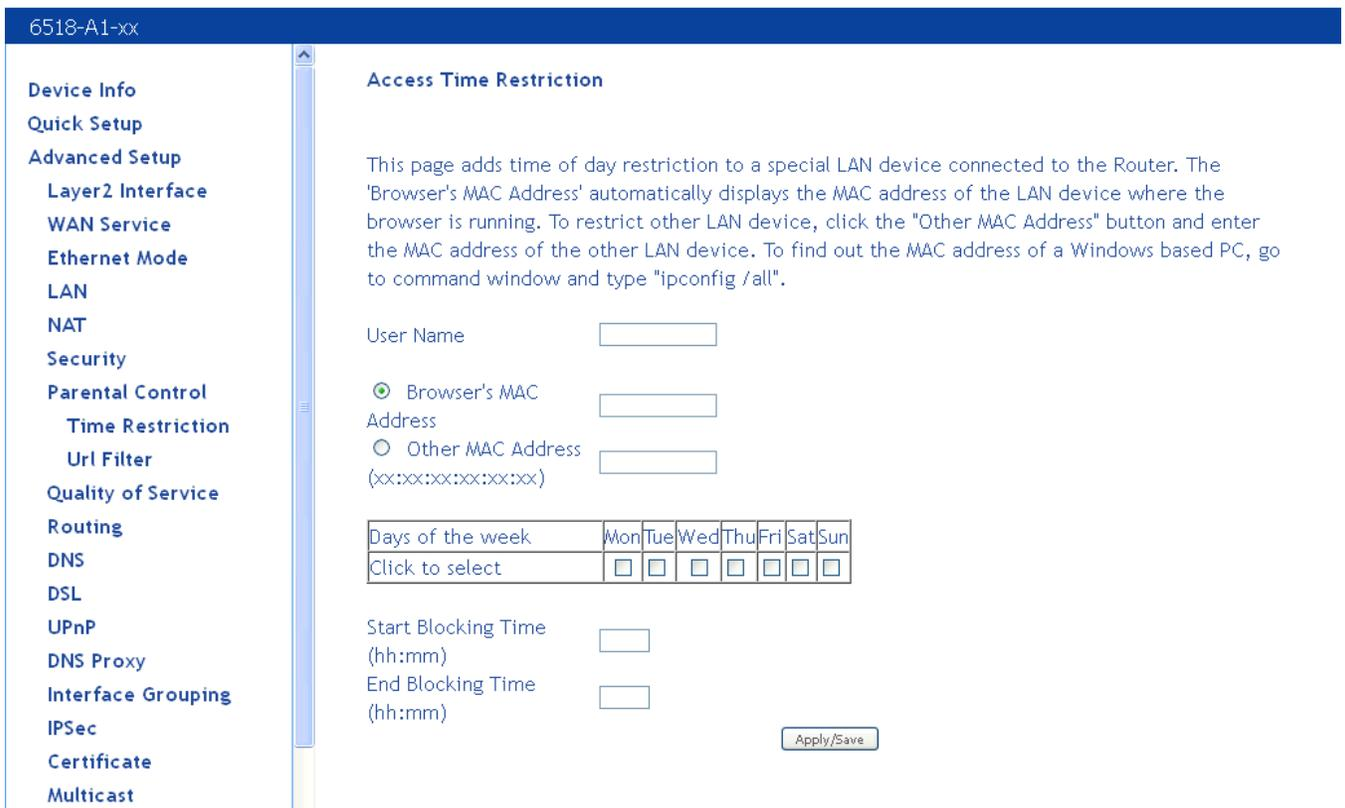
2. Enter a **User Name** to identify the target of the restrictions. . This is equivalent to the host name of the IP clients (refer to the **DHCP status** screen check to see the host names)
