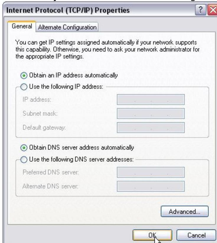
5. Or select **Use the following IP address** and enter the IP address, Subnet mask, Default gateway. Of course, you need to input the DNS server address provided by your ISP. Otherwise, you can use the ZSR4134WE's default gateway as the DNS proxy server. Click **OK** to save the configurations.
