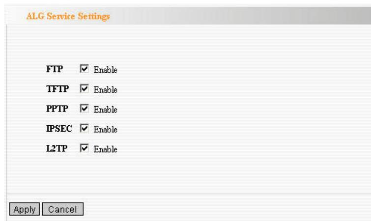
In default ALG settings, FTP/TFTP/PPTP/IPSEC/L2TP protocols are enabled. It is recommended to keep the settings unchanged.
