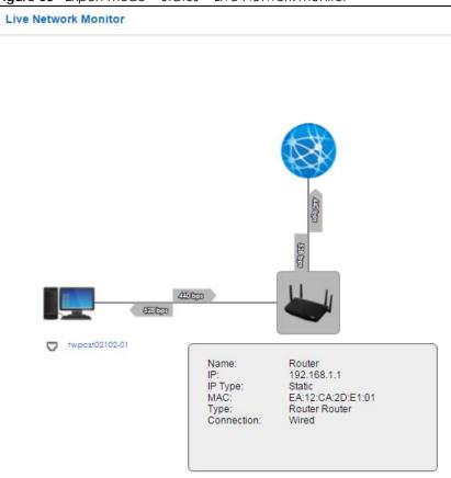
Click a device icon to go to a screen that displays the upstream/downstream bandwidth as a line graph. If you click the NBG6817's icon, it also shows the transmission rate between the NBG6817 and each connected device. If you click a connected device's icon, you can see the current transmission rate for a traffic type. The green ball indicates the traffic flow is given enough bandwidth.
