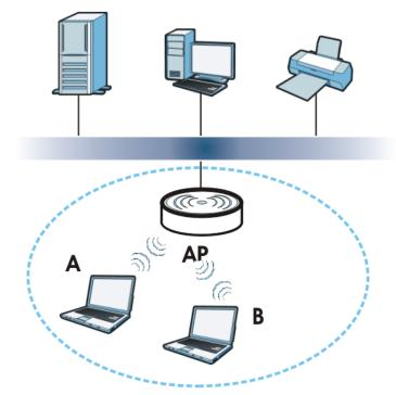
The wireless network is the part in the blue circle. In this wireless network, devices **A** and **B** are called wireless clients. The wireless clients use the access point (AP) to interact with other devices (such as the printer) or with the Internet. Your NBG6817 is the AP.
