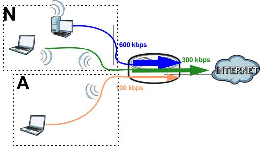
Figure 64 Example: Bandwidth for Different Networks
