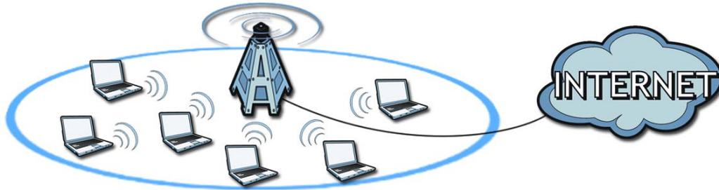
A base station's coverage area can extend over many hundreds of meters, even under poor conditions. A base station provides network access to subscriber stations and mobile stations, and communicates with other base stations.
