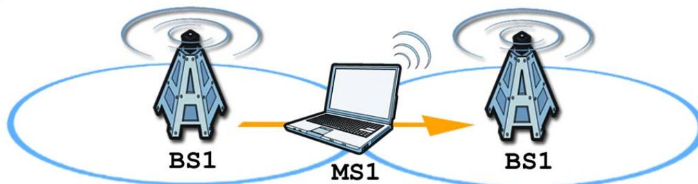
WiMAX technology uses radio signals (around 2 to 10 GHz) to connect subscriber stations and mobile stations to local base stations. Numerous subscriber stations and mobile stations connect to the network through a single base station (BS), as in the following figure.
