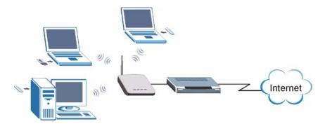
The figure below shows a network connecting to the Internet through a HomePlug connection. Select **Router(HomePlug WAN)** in the screen if you connect to the Internet as shown in the diagram.
