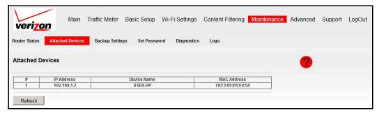
For each device, the table shows the IP address, device name if available, and the Ethernet MAC address. If the router is rebooted, this data is lost until the router rediscovers the devices. To force the router to look again for attached devices, click the **Refresh** button.
