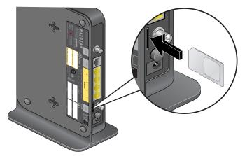
If you have not inserted the included 4G LTE SIM card into the SIM card slot on the back of the router yet, do so now.
