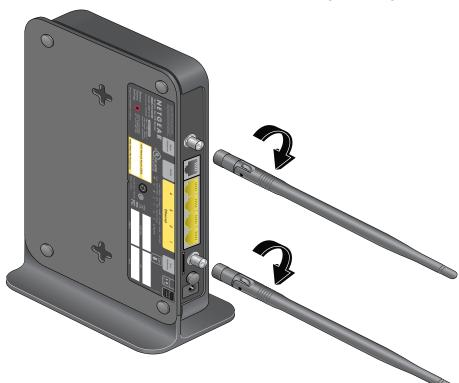
5. Install the external antennas for improved 4G LTE signal strength:
