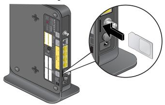
If you need to remove your SIM card from your router, gently press the SIM card inward to release it, and remove it from the slot.
