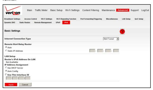
This screen specifies the remote relay router to which your router creates the 6to4 tunnel. If your ISP provides the address of its own relay router, you can put it here. You can also leave it as Auto, and the router uses any address that is available.
