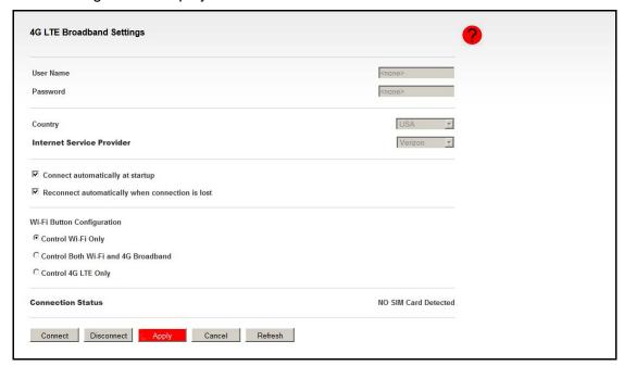
**Note:** To connect to the 4G LTE network, an active broadband service account with Verizon is required. The user name, password, country, and Internet service provider elements are not writeable or changeable. These settings are selected and provided by default when a SIM card is inserted.
