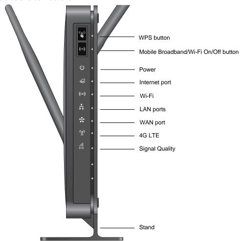
*Table 1* describes each LED and button on the front panel of the router.
