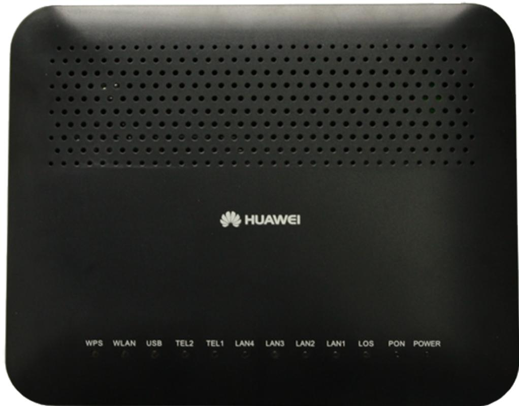
Figure 2-12 LEDs on the HG8247
