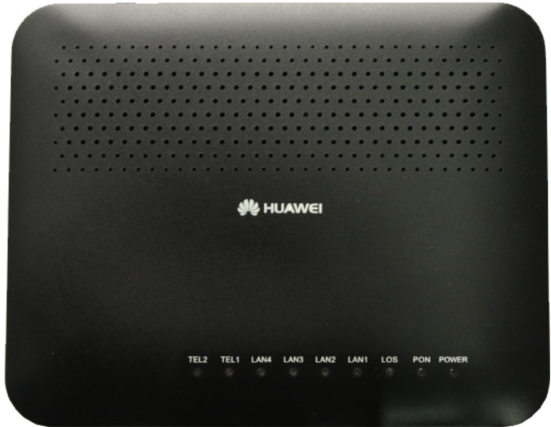
Figure 2-11 LEDs on the HG8245
