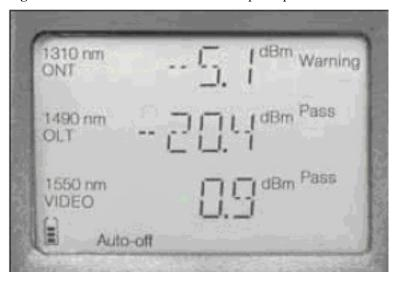
Figure 4-4 Measurement interface of the optical power meter
