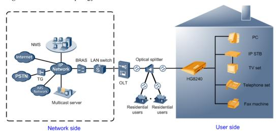
Figure 2-13 Network topology of the HG8240
