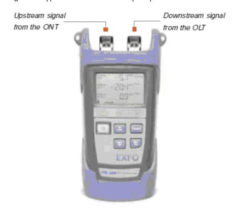
As shown in **Figure 4-2**, the PPM-350B optical power meter is different from common optical power meters. Specifically, the PPM-350B has a downstream input optical port and an upstream input optical port and can display the optical power of three wavelengths: 1310 nm, 1490 nm, and 1550 nm.
