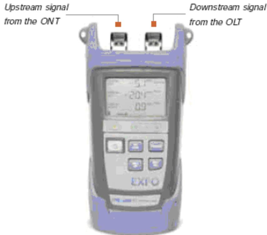
As shown in **Figure 6-2**, the PPM-350B optical power meter is different from common optical power meters. Specifically, the PPM-350B has a downstream input optical port and an upstream input optical port and can display the optical power of three wavelengths: 1310 nm, 1490 nm, and 1550 nm.
