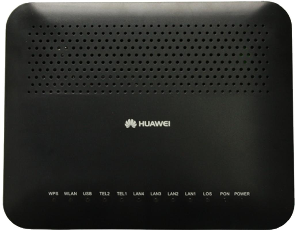
Figure 2-23 LEDs on the HG8247
