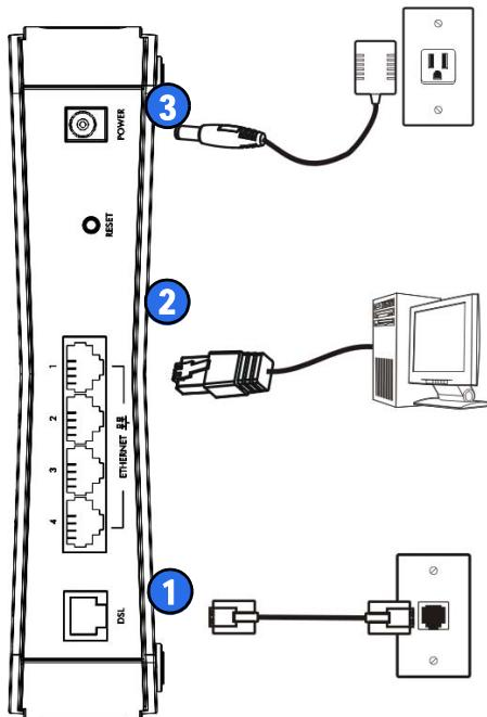
1. **DSL:** Use a telephone cable to connect your P-660HN-51's **DSL** port to a telephone jack (or to a splitter, if one is already installed).
