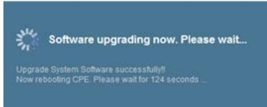
Normally, the upgrade process may take around 6 minutes for both the IDU and ODU. The login page appears again after the upgrade is done.
