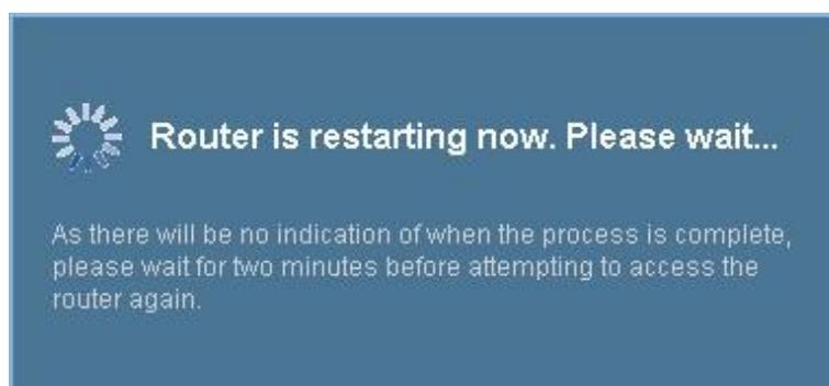
You can also press the **RESET** button on the back panel to reset the factory defaults of your LTE Device. Refer to Section 1.7 on page 6 for more information on the **RESET** button.
