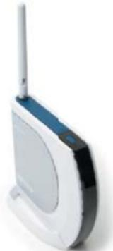
In some environments it's desirable to further increase range by installing an external, higher-gain antenna. External antennas come in all shapes and sizes. Antennas also come with different connectors. The WHR-HP-G54 has an *RP-SMA* connector on it. If your antenna has a different kind of connector, you'll need an adaptor.
