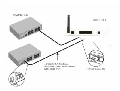
If you wish to reserve the uplink port on the switch or hub for another device, connect to any on the other MDI-X ports (1x, 2x, etc.) with a crossed cable.
