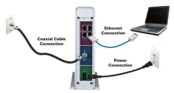
Figure 3 – SBG6782-AC Connection Diagram
